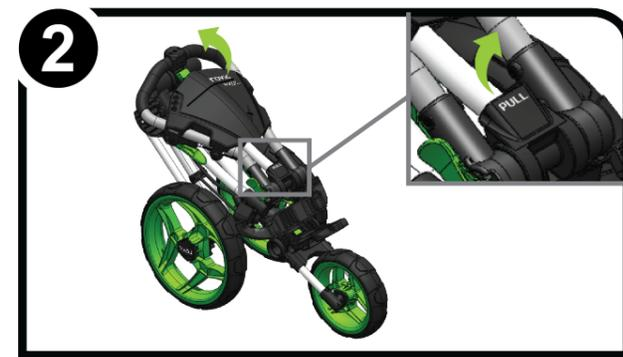
**2** USE ONE HAND TO HOLD DOWN THE LOWER PART OF THE CART AND LIFT UP THE FOLDED HANDLE USING THE "PULL" HANDLE.
